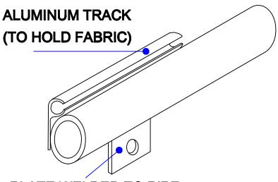
PLATE WELDED TO PIPE SPACING DETERMINED BY ENGINEER
