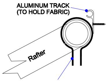
SMOOTH CLAMP AROUND PIPE SPACING DETERMINED BY ENGINEER
