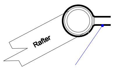
SMOOTH CLAMP AROUND PIPE SPACING DETERMINED BY ENGINEER
